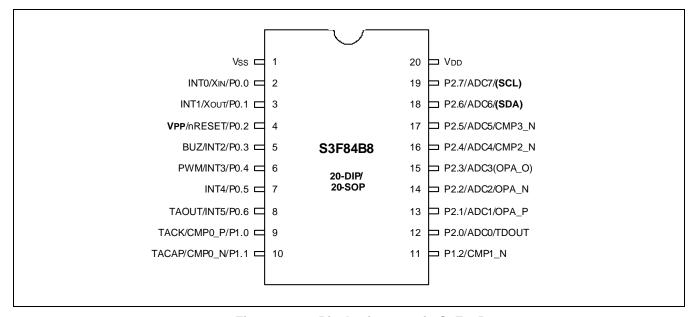
Figure 1-2 Pin Assignment in S3F84B8
